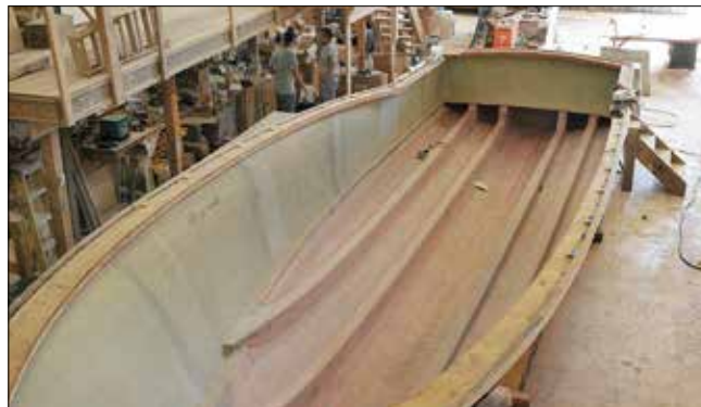
Left —Chunky longitudinal stringers of laminated Douglas-fir with sections up to 16" x 6" (406mm x 154mm) are the structural base for the cold-molded wood hulls designed by Matthews and built by F&S. Right —In this smaller 36' (11m) Matthews design, the stiff wood stringers are married to a lighter-weight foam-cored FRP hull.
