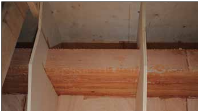
Left —Chunky longitudinal stringers of laminated Douglas-fir with sections up to 16" x 6" (406mm x 154mm) are the structural base for the cold-molded wood hulls designed by Matthews and built by F&S. Right —In this smaller 36' (11m) Matthews design, the stiff wood stringers are married to a lighter-weight foam-cored FRP hull.
