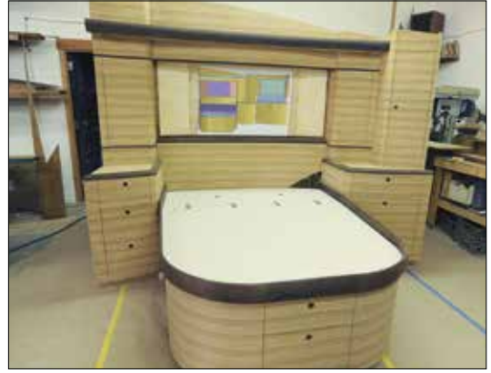
In the finished hull F&S installs complex systems and the interior joinery of the client's choice. Left —The big diesels that power these boats are firmly affixed to the structural fir stringers so prominent in the build photographs. Right —A mock-up of a master stateroom assembly.
