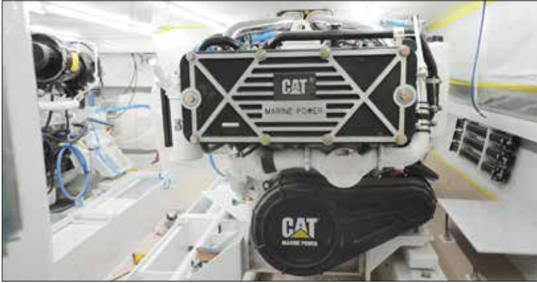
In the finished hull F&S installs complex systems and the interior joinery of the client's choice. Left —The big diesels that power these boats are firmly affixed to the structural fir stringers so prominent in the build photographs. Right —A mock-up of a master stateroom assembly.
